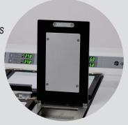
Lid heaters: This newly added lid heaters promise the temperature in the chambers even more stable. Works great with the pre-heated gas mixture for bertter uniformed temperature control.
